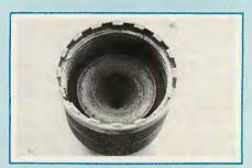
Inside view of silencer's rear nut shows elastomer wipe which limits gas escape, but ruins accuracy.
